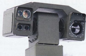
The mast-mounted electro-optical system of the A32 combat module combines daylight television, a thermal camera and a laser rangefinder. Miroslav Gyürösi: 1331767
