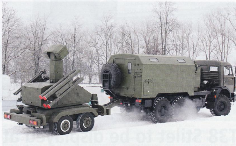
A missile-armed A32 combat module is towed by the A31 command post. Miroslav Gyürösi: 1331766
