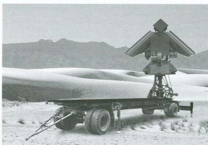
> The new phased-array command-guidance antenna mounted at the top of the trailer-mounted UNV-2TM antenna unit is smaller than the original parabolic antenna.
